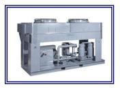
Cooling Technology's Integrated Air-Cooled Chillers feature scroll, reciprocating or screw compressors paired with a stainless steel brazed plate evaporator and an optional integral insulated stainless-steel reservoir with a non-ferrous pump. These chillers are designed for outdoor locations with low ambient controls to 0°F with optional -20°F capability. ICA line of chillers are available in 15 to 160 ton capacities with an operating range from +65°F to -30°F.
